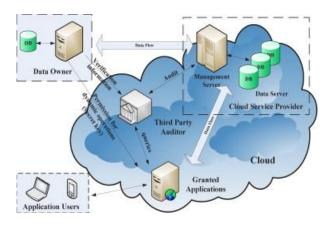
Fig 1: Cloud data storage architecture
